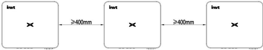
Fig 4.5 side by side installation spacing requirements
